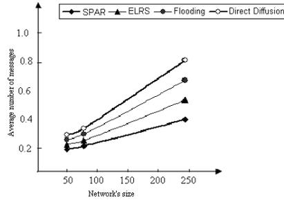
Fig. 3: increment size of network and average number of messages
